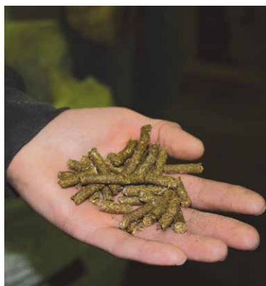
Pellets made from a mixture of cattails and prairie grasses help heat the Living Prairie Museum.
